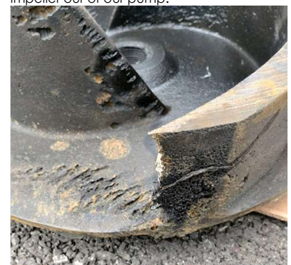
Pictured below: the recently damaged impeller out of our pump.
