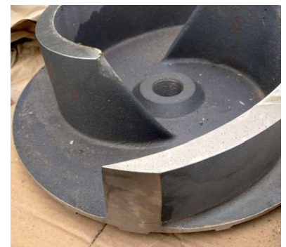
Pictured above: a brand new impeller for a sewer pump.
